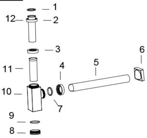
Adjust height of tubes (2) and (11) to required height to meet basin waste and align with main waste pipe, then secure nut (3).
